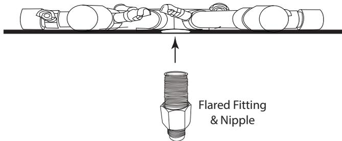
**Fig. 4** Installing nipple into bottom of burner.
