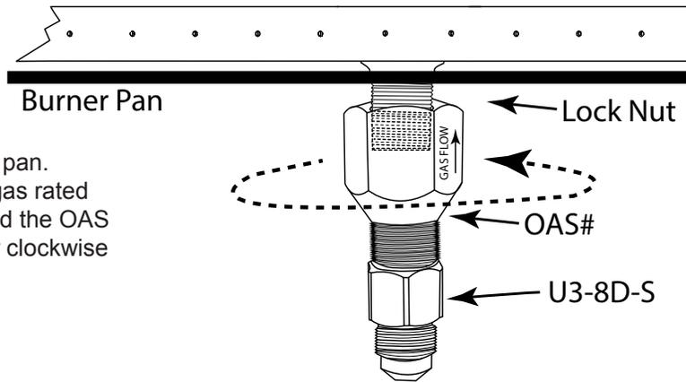
Fig. 5 Installing OAS (orifice) to burner tube.
