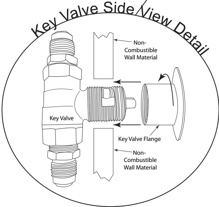
**Note:** A 1¼" x 2" black iron or galvanized coupler/nipple (not supplied) can be used as a spacer between the manual valve and the valve flange to add additional support to hold the manual key valve in place.
