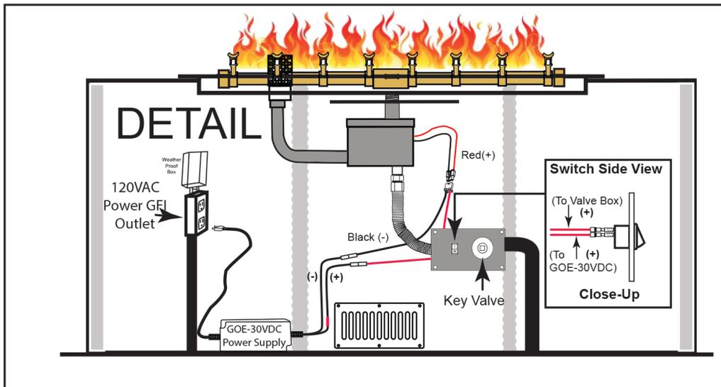
**Fig. 7** Example of a single fire feature install with power supply and switch contained within the enclosure, when applicable. **Note:** Must be 10-feet or more from a pool/spa for this installation. See additional illustration on page 10, Fig. 8.
