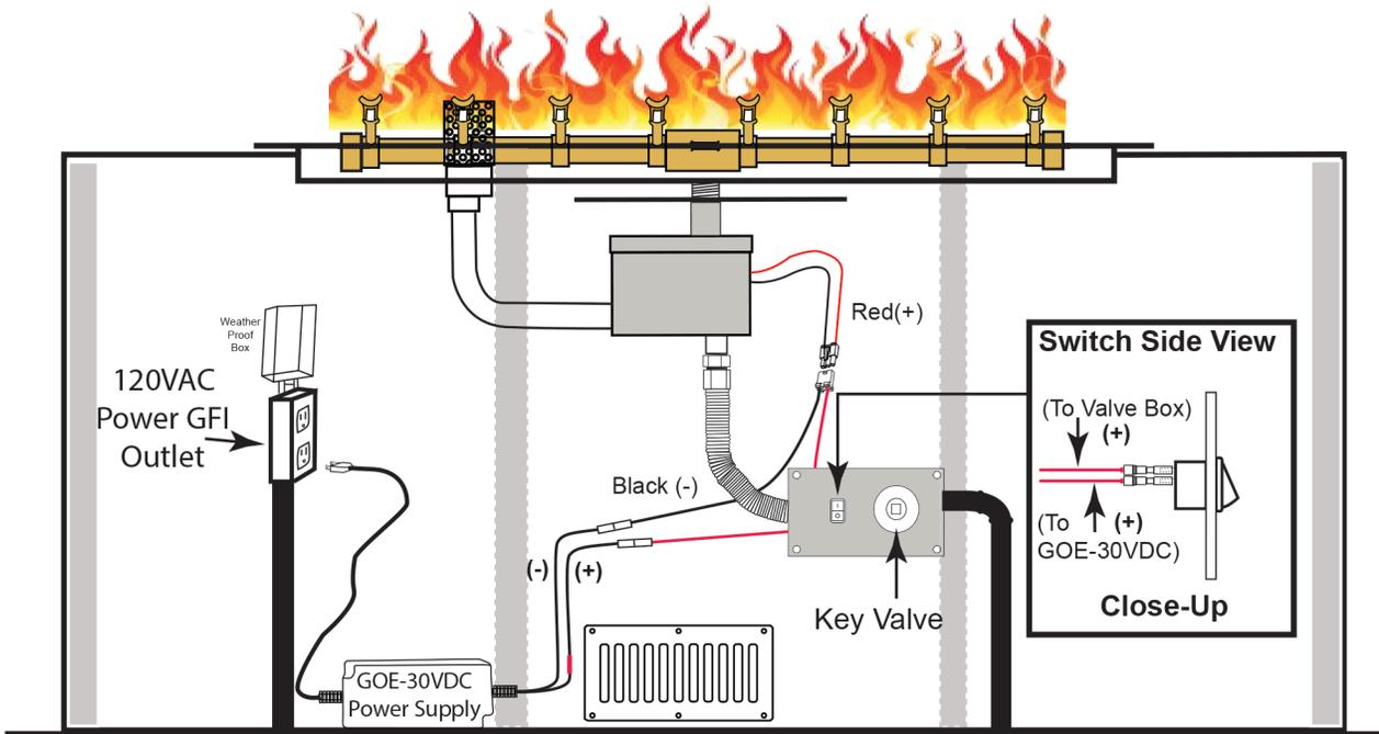
Fig. 8 Show typical wiring diagram with switch.
