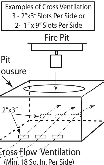
**Fig. 3** Shows cross ventilation in a enclosure.
