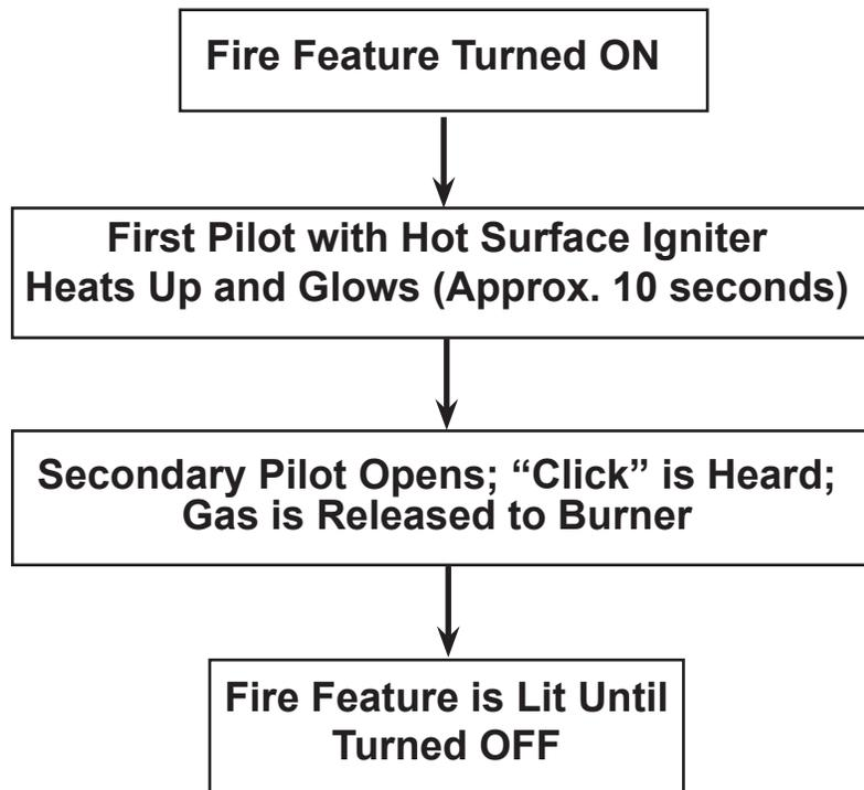
The system is designed to relight itself if blown out. It will try (3) times to relight before it goes into a "hard" lock out. Then it must be turned OFF and back ON to reset it .
