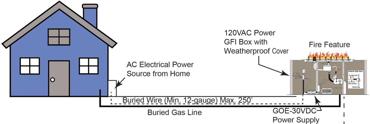
**Note:** The GOE-30VDC power supply is rated for outdoor applications and is suitable for damp dry locations and can sit on the floor of the enclosure.
