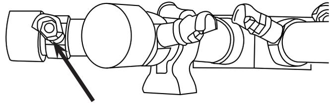
Fig. 6 Arrow shows one injector with brass cap/cover.
