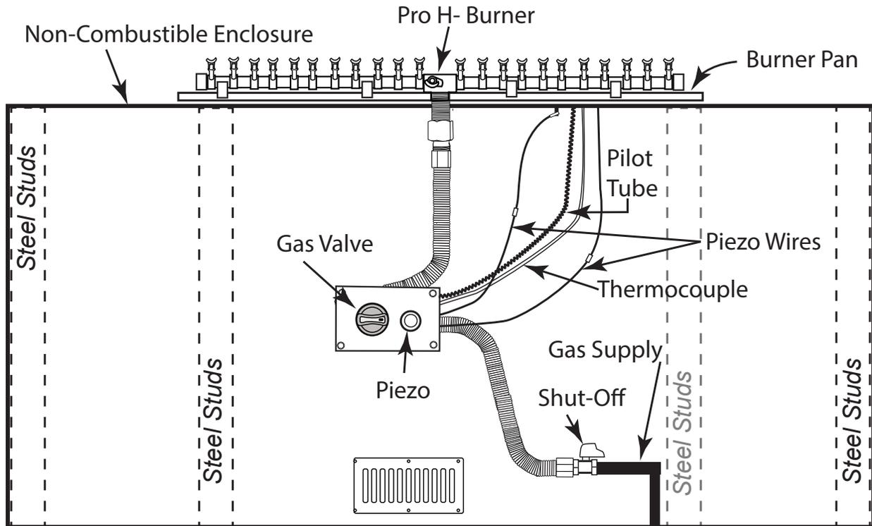
Gas valve and flexible gas lines are supplied; E-Stop shut-off is not supplied, but available in accessories page. Flex lines with flared fittings do not require Teflon tape or pipe compound. Ensure not to “kink” the flex lines to allow better gas flow of gas. The illustration above is only a guide for the gas connection. Local codes may require different methods to connect the gas supply. **Note: See optional mounting method of TPSI face plate on back of this manual.**
