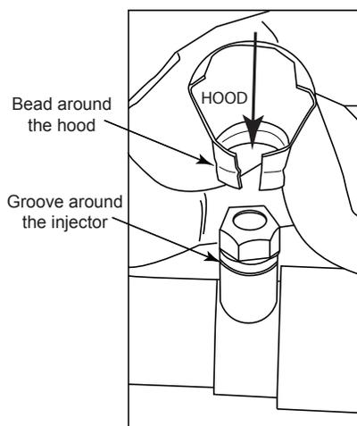
**Fig. 10** Installing hood over top of injector.
