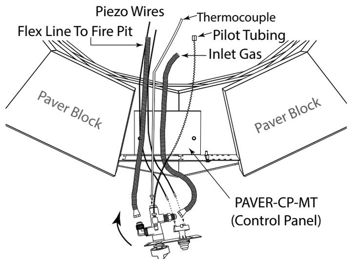
**Fig. 5** Installing control panel into PAVER-CP-MT mounting plate.
