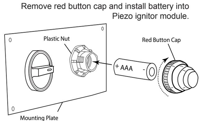
Fig. 7 Installing battery into Piezo.
