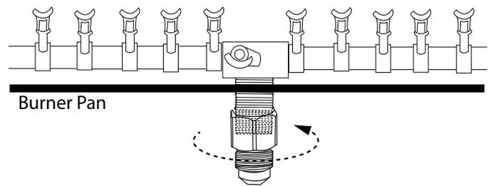
**Fig. 4** Installing nipple into bottom of burner.
