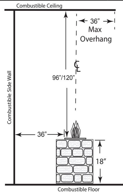
**Fig. 2** Clearance to Combustibles for models.
