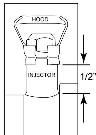
**Fig. 11** Shows 1/2” spacing from bottom of injector.
