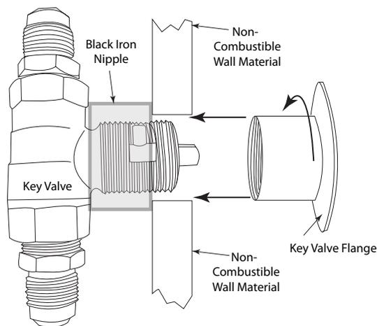
Fig. 7 Typical installation.
