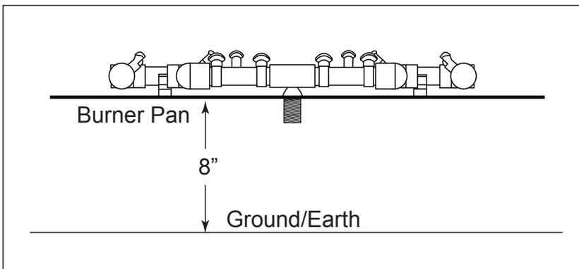
**Fig. 1** Snowflake style flat burner pan clearance specifications.
