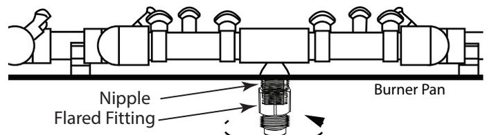
**Fig. 5** Installing gas line to Pro Burner.
