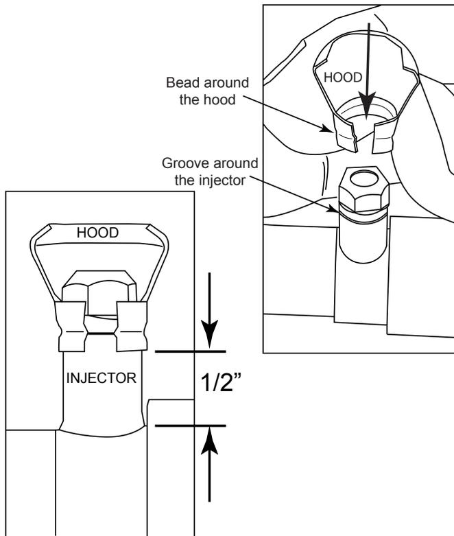
Fig. 8 Installing injector hoods.
