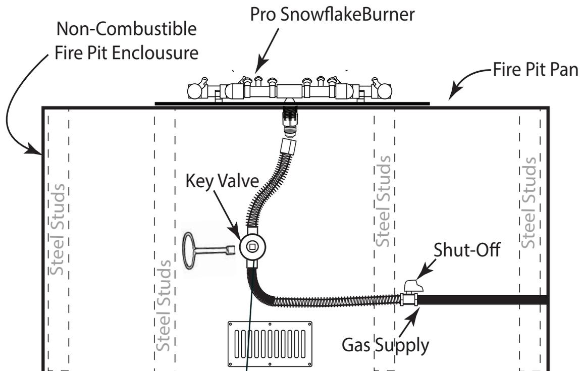
Key valve and flexible gas lines are supplied. Flex lines with flared fittings do not require Teflon tape or pipe compound. Ensure not to “kink” the flex lines to allow better gas flow of gas. The illustration above is only a guide for the gas connection. Local codes may require different methods to connect the gas supply.
