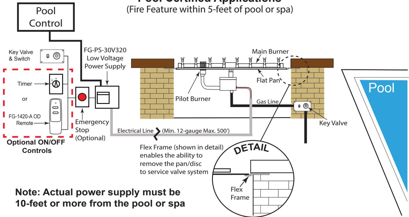
Fig. 6 Shows any fire feature installed within 5 feet of a pool or spa requires FG-PS-30V320 power supply (purchased separately). **DO NOT USE THE GOE-30VDC.** FG-PS-30V320 power supply can be installed up to a maximum of 500-feet away from fire pit.
