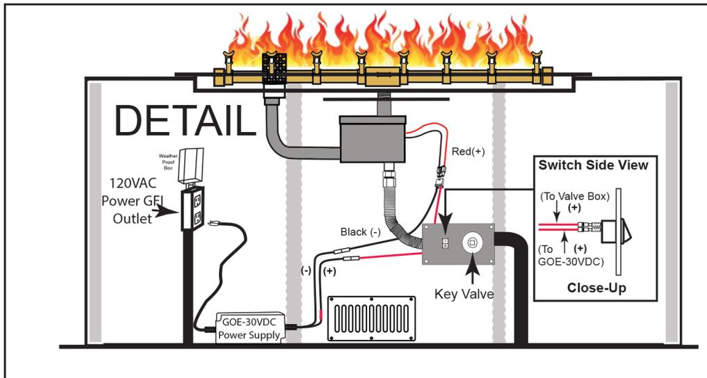
**Fig. 4** Example of a single fire feature install with power supply and switch contained within the enclosure, when applicable.
