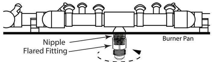
**Fig. 5** Installing gas line to Pro Burner.
