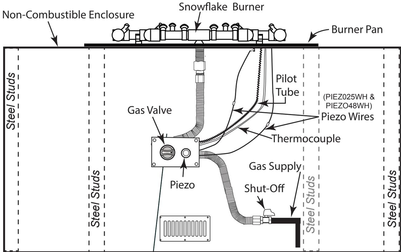
Gas valve and flexible gas lines are supplied; E-Stop shut-off is not supplied, but available in accessories page. Flex lines with flared fittings do not require Teflon tape or pipe compound. Ensure not to "kink" the flex lines to allow better gas flow of gas. The illustration above is only a guide for the gas connection. Local codes may require different methods to connect the gas supply. **Note: See optional mounting method of TPSI face plate on back of this manual.**
